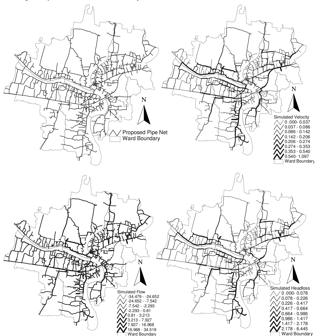
Figure 6 Simulated velocity, flow and headloss in proposed distribution network of Lohagara Municipality
